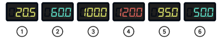
The ITP-17 indicator setup allows for the configuration of any user-defined color change thresholds and the corresponding colors within the signal measurement range. The only rule is that the threshold values for each subsequent color zone must be greater than the previous threshold.
